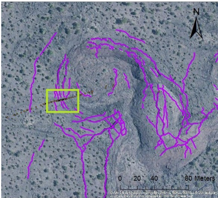
Figure 2. The graph contains the DGPS points for Traverse K, an example of a Type B crack pattern escarpment. In the graph, the blue diamonds are DGPS points and the red squares are crack markers (usually on either side of a crack, but occasionally only one point per crack). The lower picture is a satellite image of the escarpment that Traverse K crossed. The green box highlights the slope, the magenta lines denote the largest, and most visible cracks. The dark blue dots on the slope are the Traverse K DGPS points.
