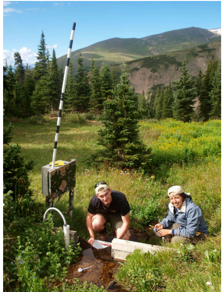
Figure 5. Claudia Corona and Ian Nesbitt measuring discharge and sampling water chemistry, Saddle Stream, Green Lakes Valley.
